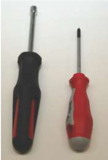
Figure 8.1a .25-inch hexnut screwdriver and Phillips-head screwdriver
