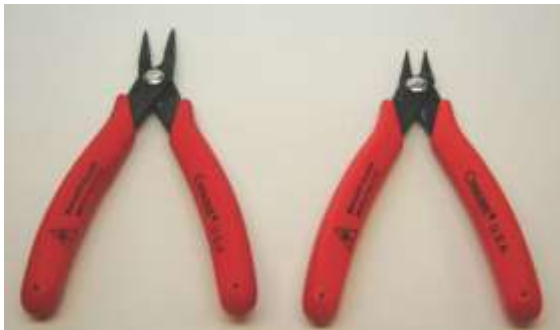
Figure 8.1d needle nose pliers and side cutters
